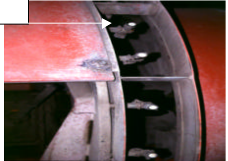
Figure 1b. Close-up of high-pressure nozzles in back of tank that sprayed the pesticide mixture up into the air
