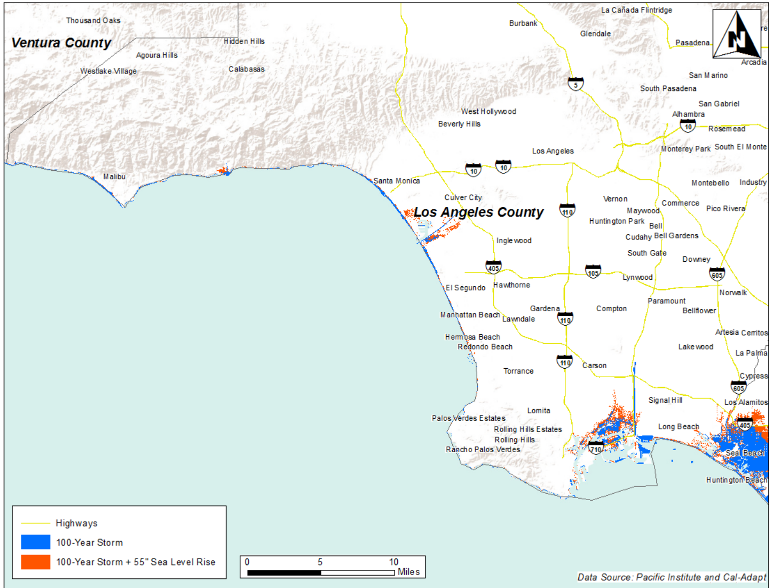
Figure 5. Baseline inundation areas for a 100-year flood (2000) and modeled scenario with additional 55 inches of sea level rise (2100), Los Angeles County 6 Note: Current projections are 66 inches above sea level. 7
