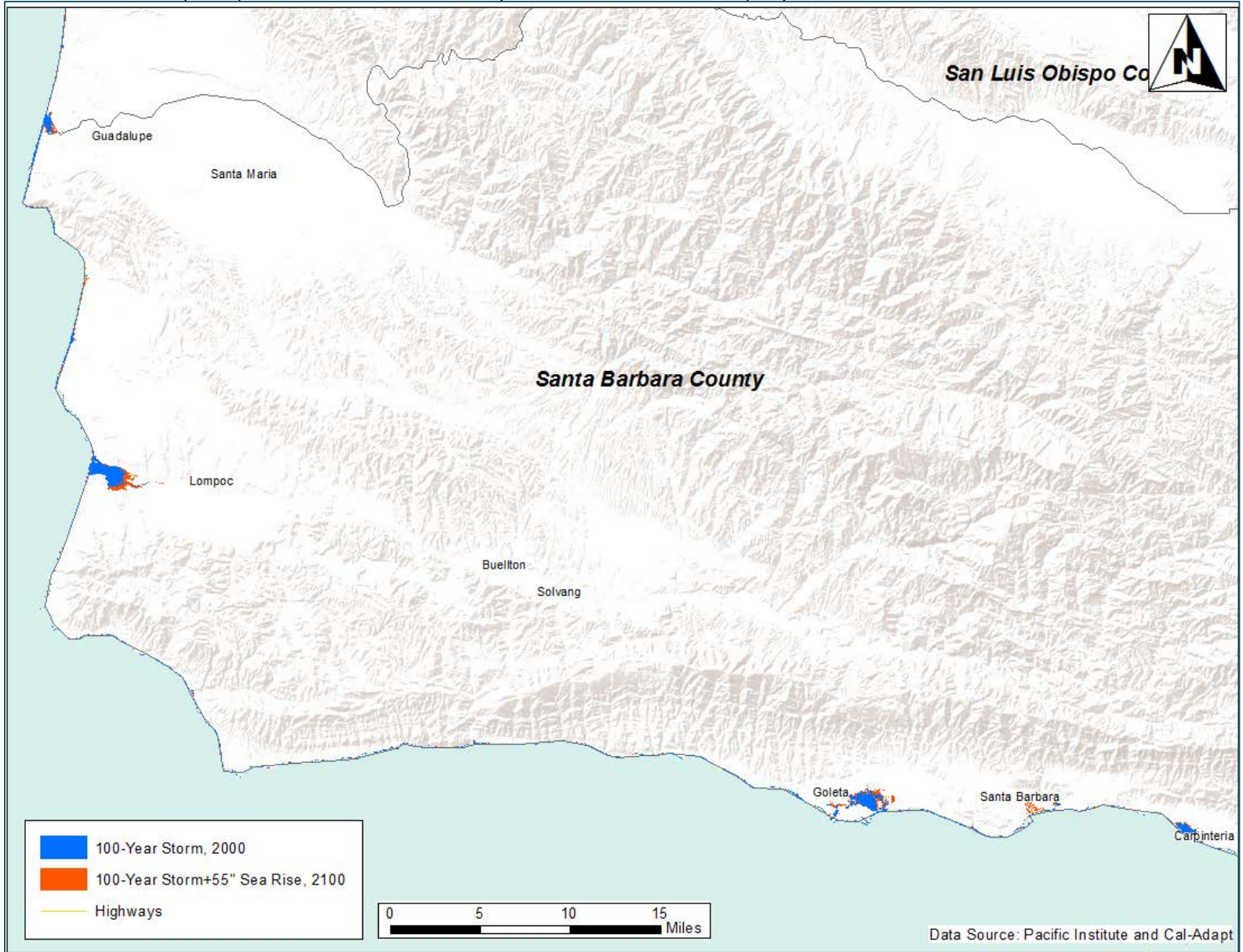
Figure 5. Baseline inundation areas for a 100-year flood (2000) and modeled scenario with additional 55 inches of sea level rise (2100), Santa Barbara County 6 Note: Current SLR projections are 66 inches above sea level. 7
