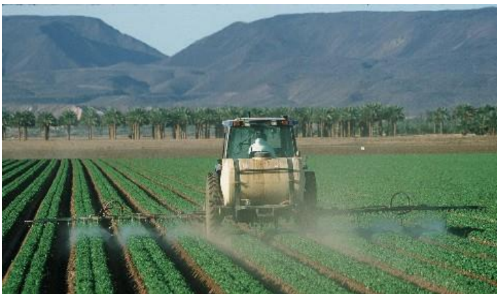
Boom sprayer being used to apply pesticides to a field. Photo courtesy of USDA NRCS
